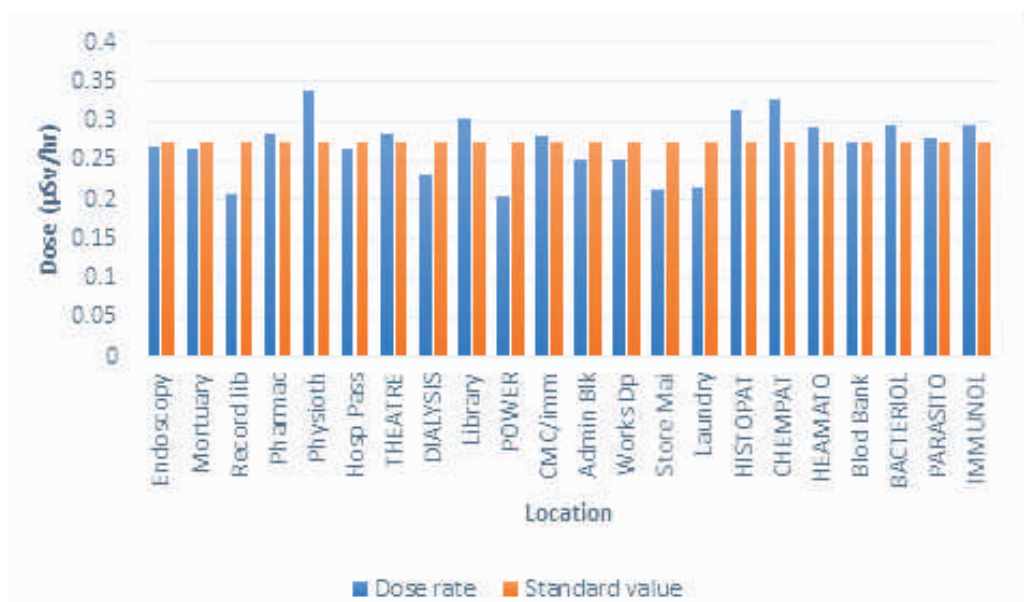
Fig. 4: Laboratories and other locations dose rate compared to the standard value.
